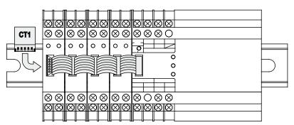
The 'Control Bus' straps on each extender unit connect to the adjacent (right hand side) module as shown.
