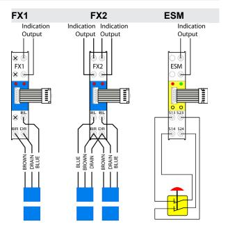
NOTE: The FX2 requires the commoning of the supply and drain wires (BROWN / DRAIN) from the two switches at the extender module as shown above.
